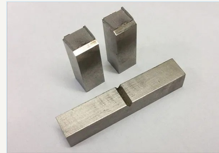
Charpy V-notch specimens — illustrative test artefact.
